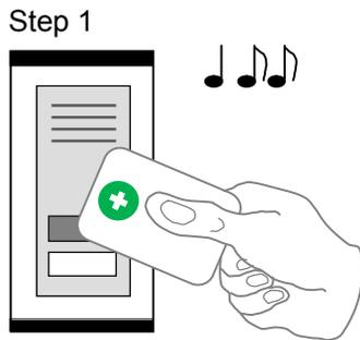
Read the programming card for *inserting*: the reader goes into *programming mode*, which is indicated by slow flashing of yellow LED.
