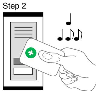
Read the programming card for inserting 5 times in a row; the reader will go into *Deleting cards "above or below"* mode indicated by fast flashing of yellow LED.
