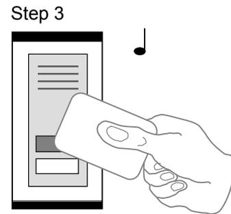
Read a card, which is located in the module's memory *right before or right after* the card you wish to delete. After this step the module quickly flashes with yellow LED.
